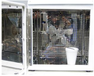
3. Place sample probe into ice bath and allow 10 - 15 seconds for sample probe temperature to stabilize.
