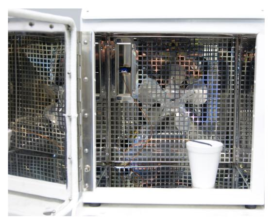
6. Remove the sample thermocouple from the ice bath, allow probe to dry before placing in a container of liquid nitrogen. Allow 10 - 15 seconds for sample probe temperature to stabilize.
