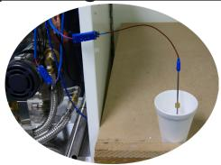
3. Place chamber probe into ice bath and allow 10 - 15 seconds for chamber probe temperature to stabilize.
