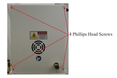
10. Replace the back cover of freezing chamber by tightening the 4 phillips head screws. [G]
