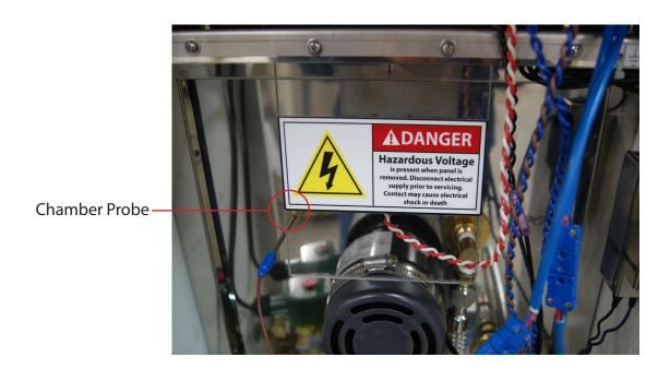
2. Locate and remove chamber probe by loosing the brass fitting using 3/8" wrench. [B]
