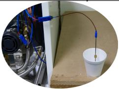
6. Remove the chamber thermocouple from the ice bath, allow probe to dry before placing in a container of liquid nitrogen. Allow 10 - 15 seconds for chamber probe temperature to stabilize.
