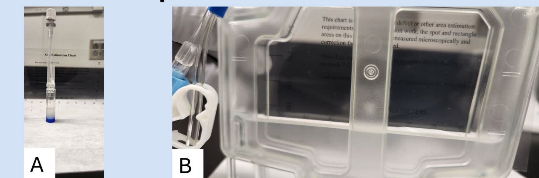
Images of TAPPI chart (A) alone, (B) viewed through a common bioprocessing container, and (C) viewed through a CryoCase. Containers are partially filled with unfiltered cell culture media containing 5% human platelet lysate. The arrow indicates the 0.2mm 2 indicator spot.
