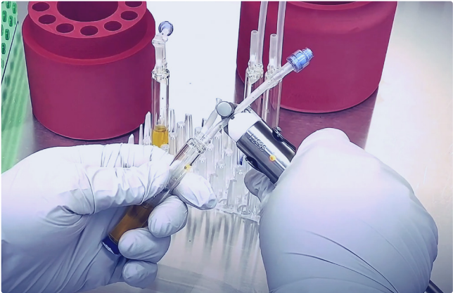
The fill line of a Needleless-Barbed CellSeal Vial is shown being sealed with the RF Tube Sealing System to ensure a solid weld and container closure integrity (CCI) for cryogenic storage. CellSeal Freezing Containers are also shown.
